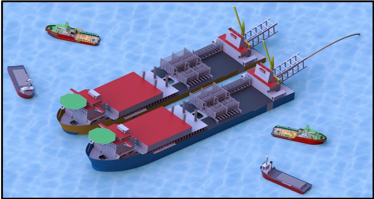
FIGURE 3: An illustrative rendering of what a skin-to-skin pipelaying configuration could look like. In such a configuration, a DPS-enabled vessel could be tethered to a pipelaying vessel without DPS, with sea-fenders deployed between the vessels while coupled. Cargo vessels would continuously deliver pipe segments to the nominal pipelayer for welding of the segments into a pipeline string, which would then be deployed in an s-lay profile to the seabed, via the ship's rear 'stinger' gantry system. Given the strong weather-sensitivity of such a configuration, support tugs would need to stand ready to pull the vessels apart should the sea state rapidly deteriorate. ( Figure for illustrative purposes only )
